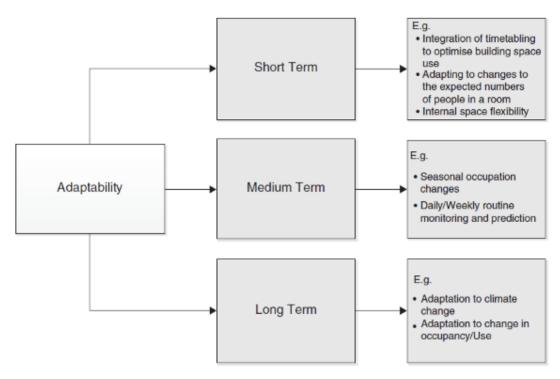
Diagram 3. Adaptability over different timescales in a Smart Building
