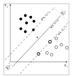
Why is it so helpful in computer vision and object detection in particular? This is due to the fact that finding the optimal division line between pixels that belong to an object and those that don't is a vital component of object detection.
