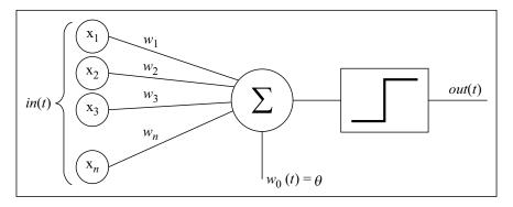
A sigmoid function is a term that indicates that the function produces either a 0 or 1 value. The discriminant is a threshold value; if the weighted sum of the inputs is greater than a certain threshold, the perceptron produces a binary classification of 1, otherwise 0.
