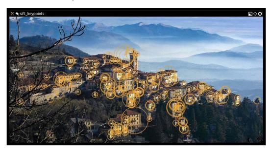
This image has been obtained by processing it with a SURF algorithm using a Hessian threshold of 8000. To be precise, I ran the following command:
