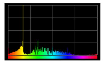
The picture shows a representation of a color histogram with one column per value from 0 to 180 (note that OpenCV uses H values 0-180. Other systems may use 0-360 or 0-255).
