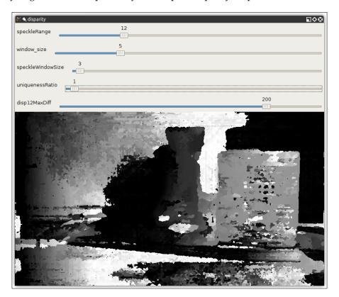
The parameters used by  ${\tt StereoSGBM}$  are as follows (taken from the OpenCV documentation):
