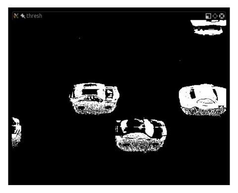
Note that shadow detection isn't absolutely perfect, but it helps bring the object contours back to the object's original shape. Let's take a look at a reimplemented example of motion detection utilizing BackgroundSubtractorKNN:
