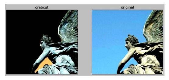
This is quite a satisfactory result. You'll notice that an area of background is left under the angel's arm. It is possible to apply touch strokes to apply more iterations; the technique is quite well illustrated in the <code>grabcut.py</code> file in <code>samples/python2</code> of your OpenCV installation.
