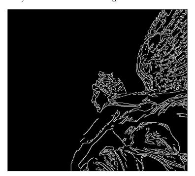
The Canny edge detection algorithm is quite complex but also interesting: it's a five-step process that denoises the image with a Gaussian filter, calculates gradients, applies **non maximum suppression** (**NMS**) on edges, a double threshold on all the detected edges to eliminate false positives, and, lastly, analyzes all the edges and their connection to each other to keep the real edges and discard the weak ones.
