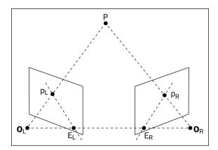
Let's see how OpenCV applies epipolar geometry to calculate a so-called disparity map, which is basically a representation of the different depths detected in the images. This will enable us to extract the foreground of a picture and discard the rest.
