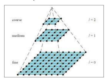
A multiscale representation of an image, or an image pyramid, helps you resolve the problem of detecting objects at different scales. The importance of this concept is easily explained through real-life hard facts, such as it is extremely unlikely that an object will appear in an image at the exact scale it appeared in our sample image.
