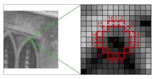
As you can see, three out of four of the test pixels (pixels number 1, 9, 5, and 13) must be within (or beyond) the threshold (and, therefore, marked as brighter or darker) and one must be in the opposite side of the threshold. If all four are marked as brighter or darker, or two are and two are not, the pixel is not a candidate corner.
