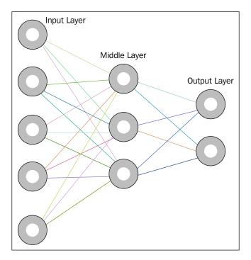
As you can see from the figure, there are three distinct layers in a neural network: **Input layer**, **Hidden layer** (or middle), and **Output layer**.
