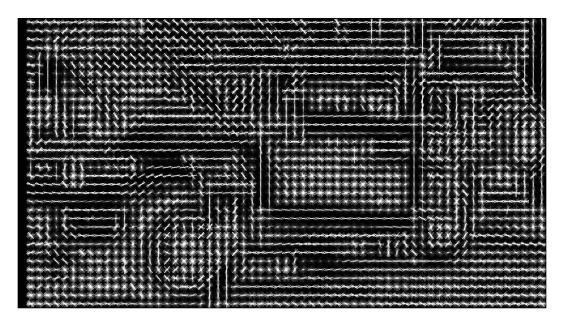
You can easily recognize the wheels and the main structure of the vehicle. So, what is HOG *seeing*? First of all, you can see how the image is divided into cells; these are 16x16 pixels cells. Each cell contains a visual representation of the calculated gradients of color in eight directions (N, NW, W, SW, S, SE, E, and NE).
