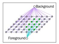
7. After the nodes have been connected to either terminal (background or foreground, also called a source and sink), the edges between nodes belonging to different terminals are cut (the famous cut part of the algorithm), which enables the separation of the parts of the image. This graph adequately represents the algorithm:
