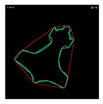
As you can see, the convex hull surrounds the entire subject, the approximated polygon is the innermost polygon shape, and in between the two is the original contour, mainly composed of arcs.
