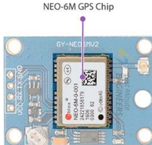
Gambar 1. Neo-6m GPS Chip
