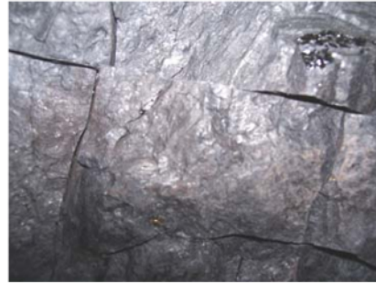
Figure 2 Coal sample showing Butt Cleats and Face Cleats
