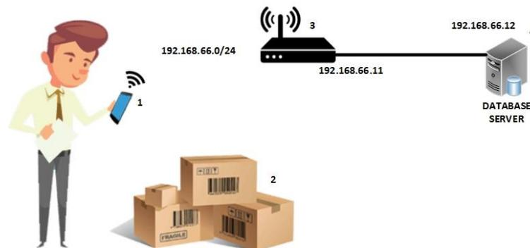
**Figure 3.** Mobile POS using Android OS smartphone.
