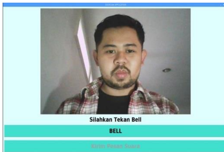
Figure 3. The Interface on LCD Monitor Telling Guest to Push the Button to Inform the Homeowner.
