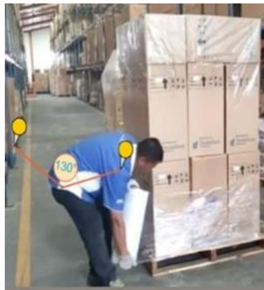
Fig. 3. Lower Wrapping Position
