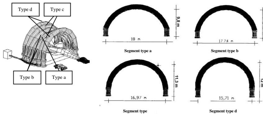
**Fig. 1. The shape and size of the building segments.**
