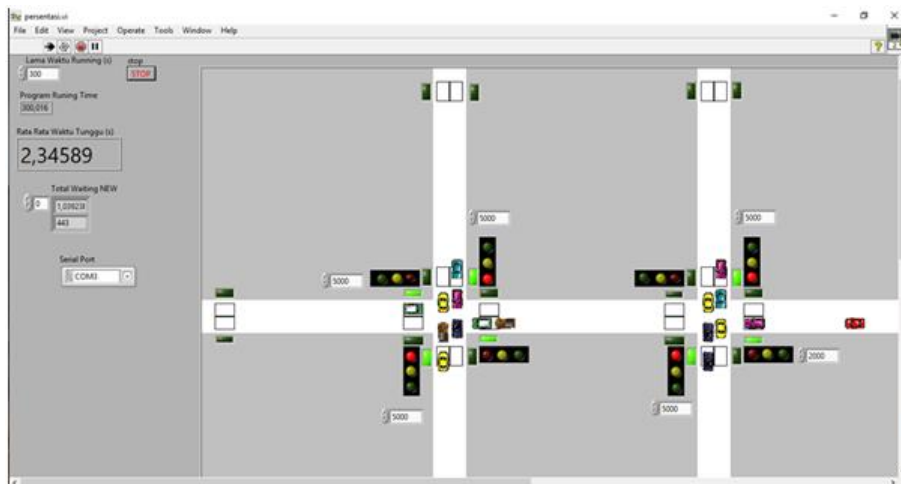
Figure 7. The GUI of the traffic light control system simulator of two adjacent intersections
