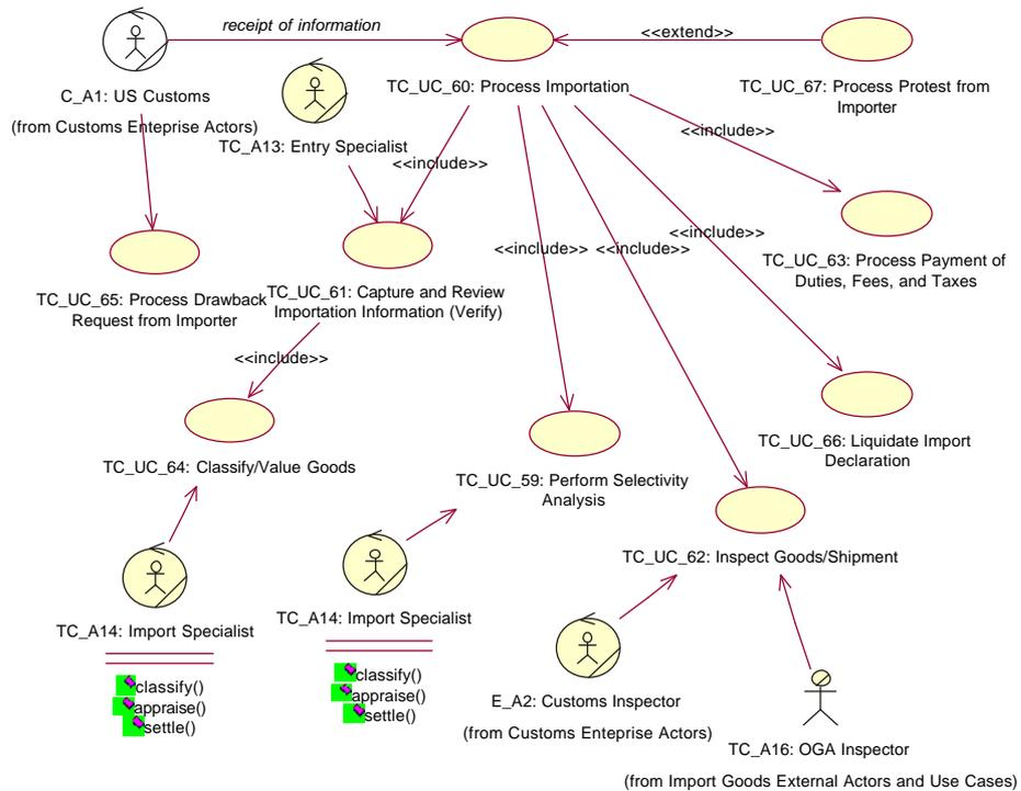
**Figure 27. Use Case Diagram, Trade Compliance Business Process—Internal**
