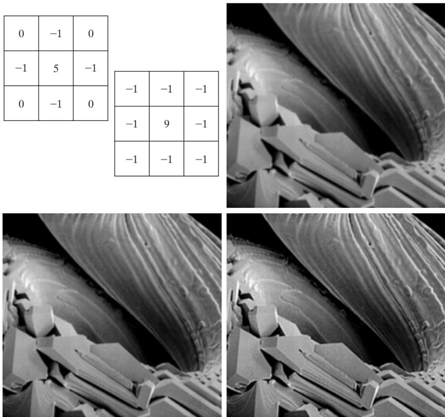
**FIGURE 3.41** (a) Composite Laplacian mask. (b) A second composite mask. (c) Scanning electron microscope image. (d) and (e) Results of filtering with the masks in (a) and (b), respectively. Note how much sharper (e) is than (d). (Original image courtesy of Mr. Michael Shaffer, Department of Geological Sciences, University of Oregon, Eugene.)
