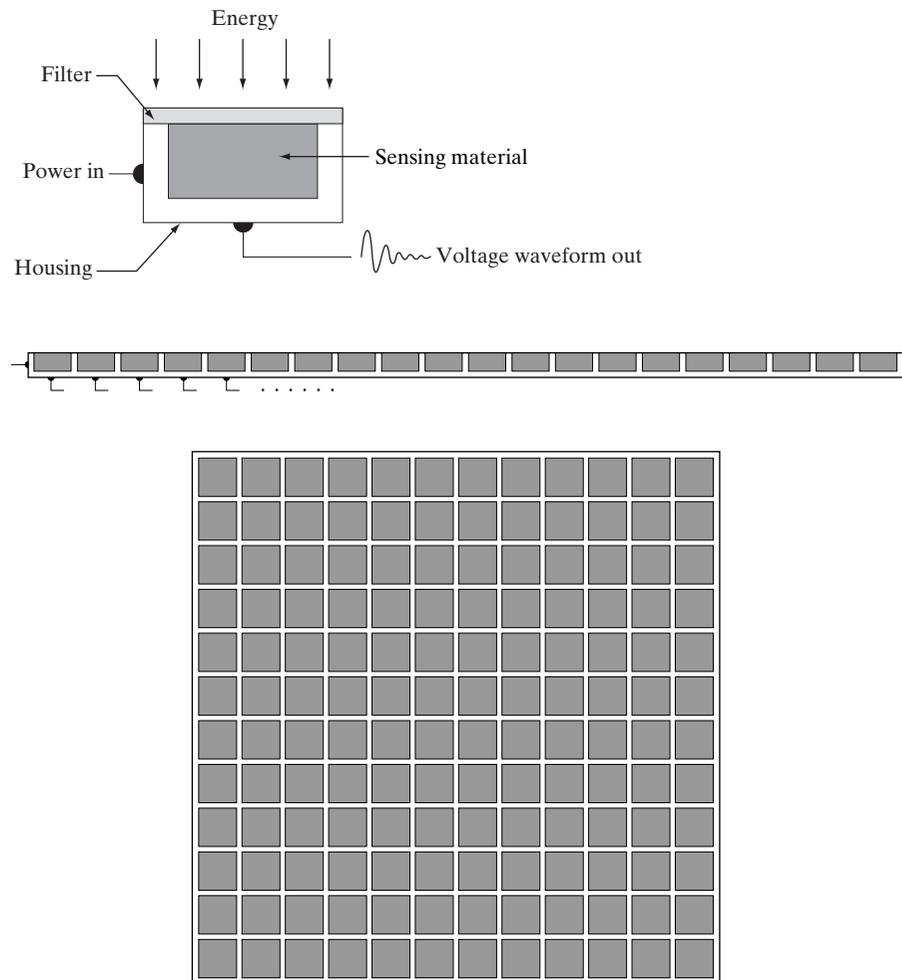
transformed into a voltage by the combination of input electrical power and sensor material that is responsive to the particular type of energy being detected. The output voltage waveform is the response of the sensor(s), and a digital quantity is obtained from each sensor by digitizing its response. In this section, we look at the principal modalities for image sensing and generation. Image digitizing is discussed in Section 2.4.
