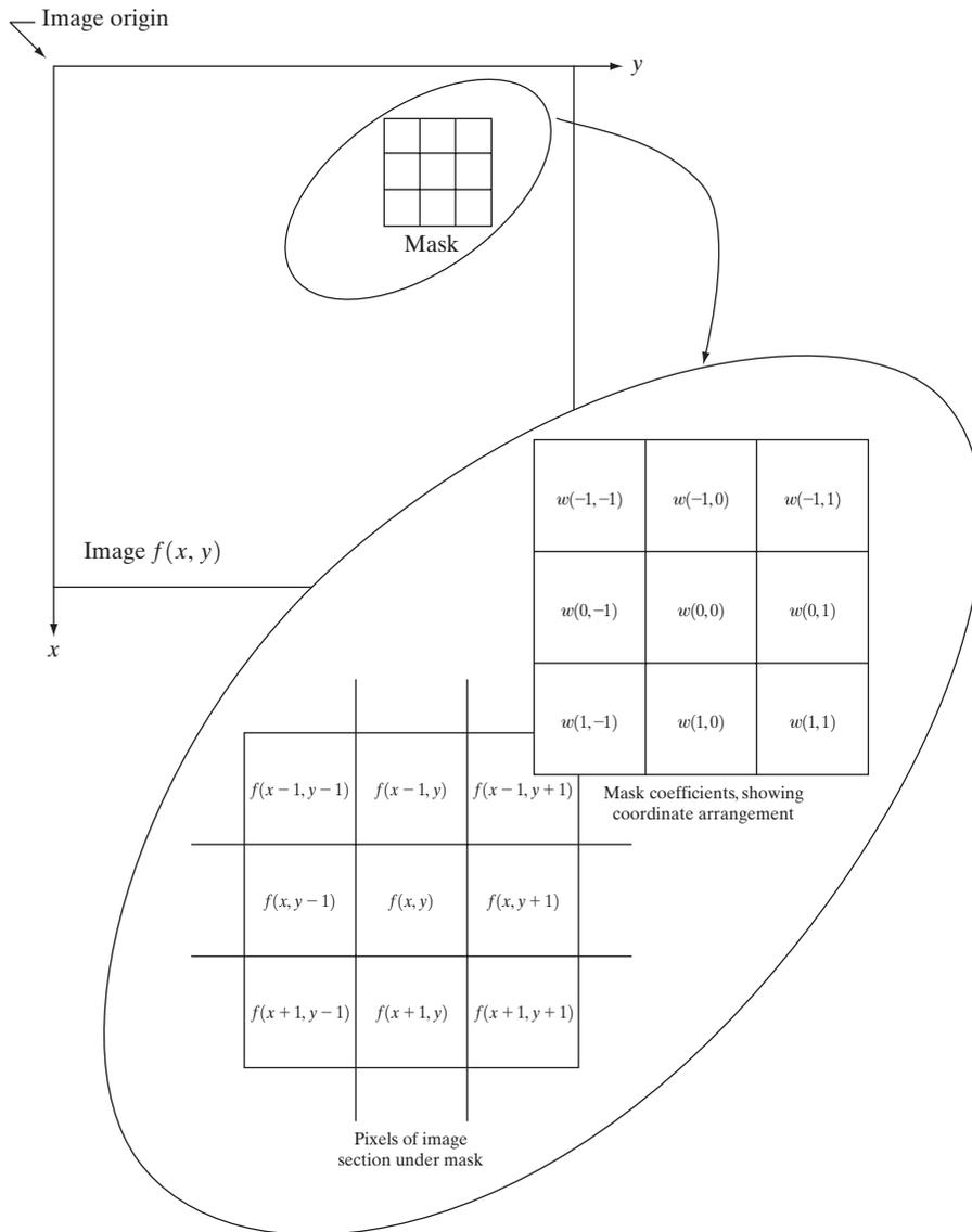
**FIGURE 3.32** The mechanics of spatial filtering. The magnified drawing shows a  $3 \times 3$  mask and the image section directly under it; the image section is shown displaced out from under the mask for ease of readability.
