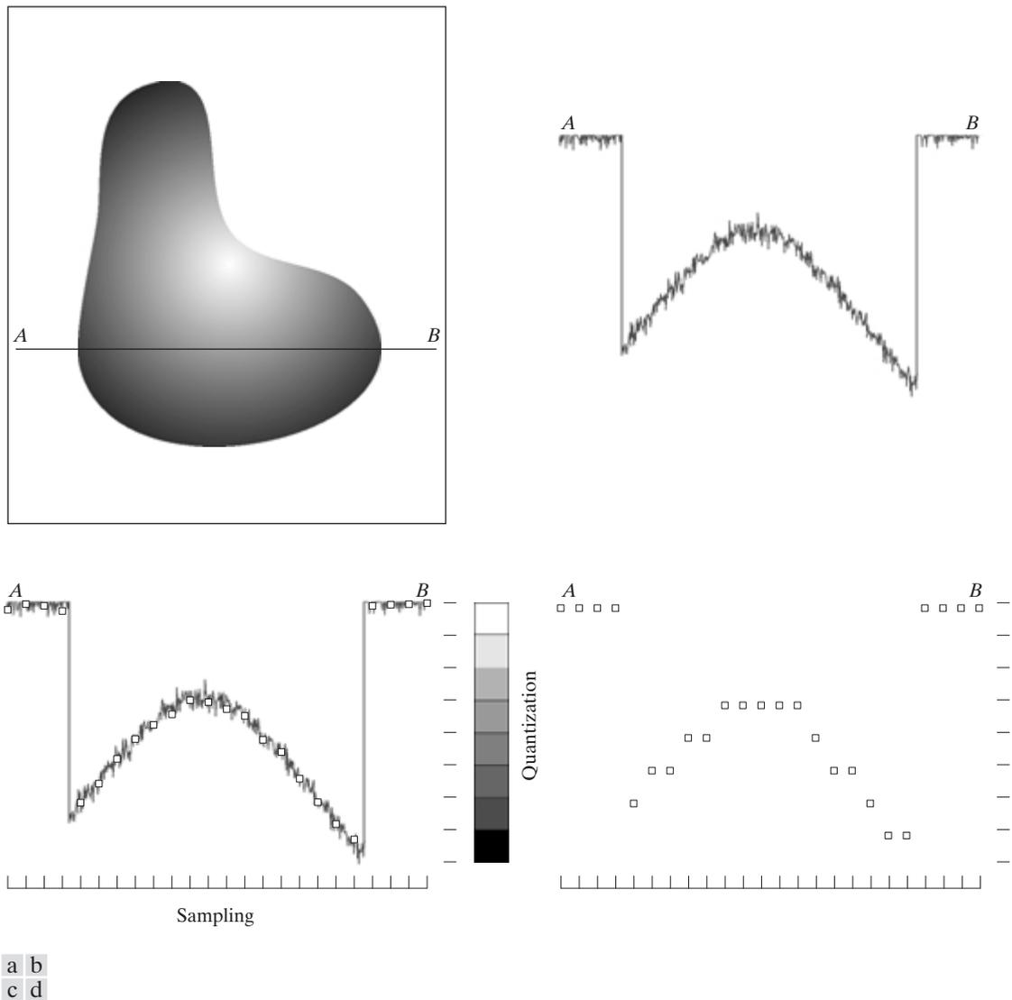
**FIGURE 2.16** Generating a digital image. (a) Continuous image. (b) A scan line from *A* to *B* in the continuous image, used to illustrate the concepts of sampling and quantization. (c) Sampling and quantization. (d) Digital scan line.
