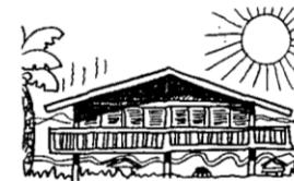
In tropical regions where it is hot and humid walls become open screens to let air pass through but keep out the heat. Verandahs and roof overhangs provide shaded outdoor "rooms".
