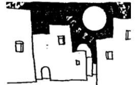
At night the heat retained in the thick walls is given off to compensate for the cooler temperature.
