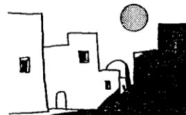
In hot dry areas thick walls keep out the heat by day, light colours reflect the sun's rays and small windows minimise glare.
