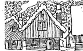
Where it is cold and wet thick dark walls of brick or wood both keep out the cold and store heat. As the sky is less bright, larger windows are needed.
