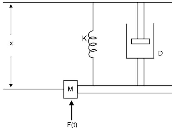
**Fig. 1.2:** Suspended weight attached with spring and piston.
