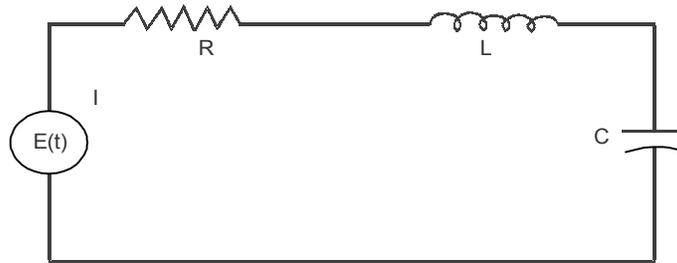
**Fig. 1.3:** Static circuit of an electrical system.
