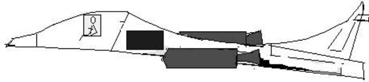
**Fig. 3.3:** Redundant components with no overlap.
