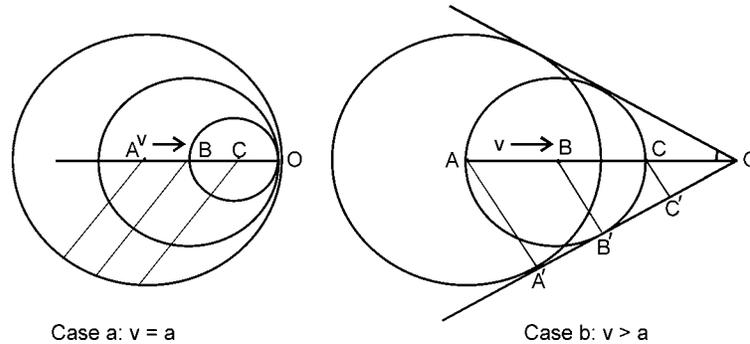
**Fig. 5.4:** Disturbance due to a body moving with sonic and supersonic velocity.
