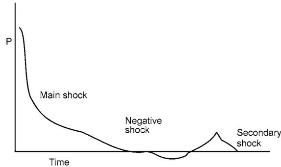
**Fig. 5.3:** Shock pressure record taken from oscilloscope.
