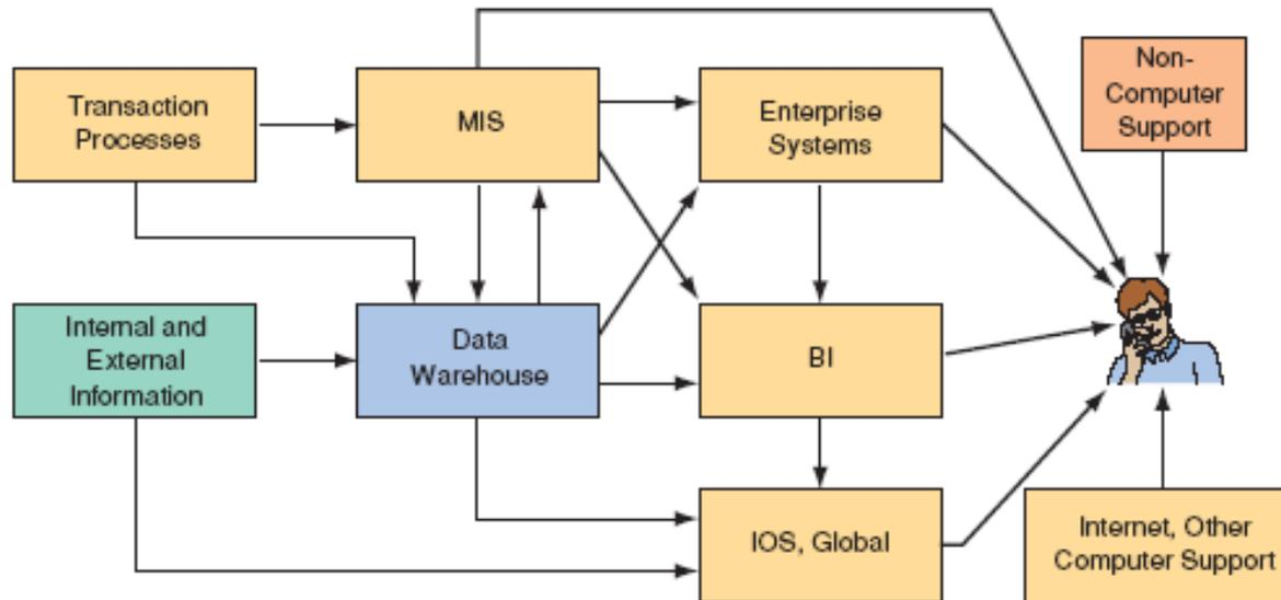
**Interrelated support systems. The TPS collects information that is used to build the MIS and the data warehouse. These feed the BI and other enterprise systems.**
