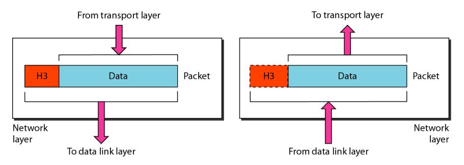
The network layer is responsible for the delivery of individual packets from the source host to the destination host.
