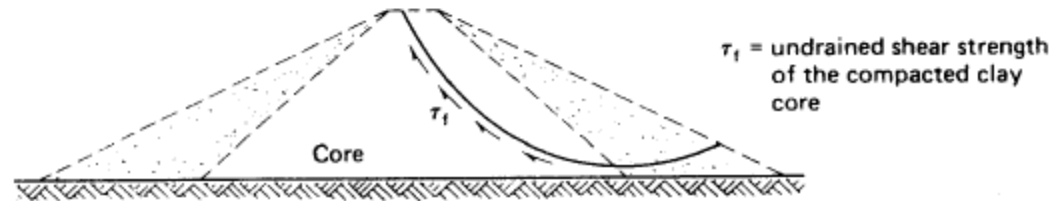
(b) Large earth dam constructed rapidly with no change in water content of clay core
