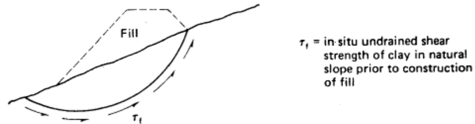
(c) Rapid construction of an embankment on a natural slope.
