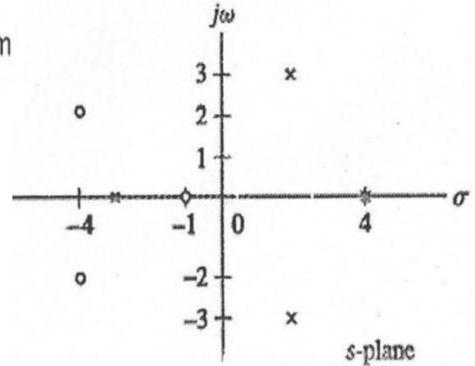
$$X(s) = \frac{a_0 s^m + a_1 s^{m-1} + \dots + a_m}{b_0 s^n + b_1 s^{n-1} + \dots + b_n} = \frac{a_0 (s - z_1) \dots (s - z_m)}{b_0 (s - p_1) \dots (s - p_n)}$$
