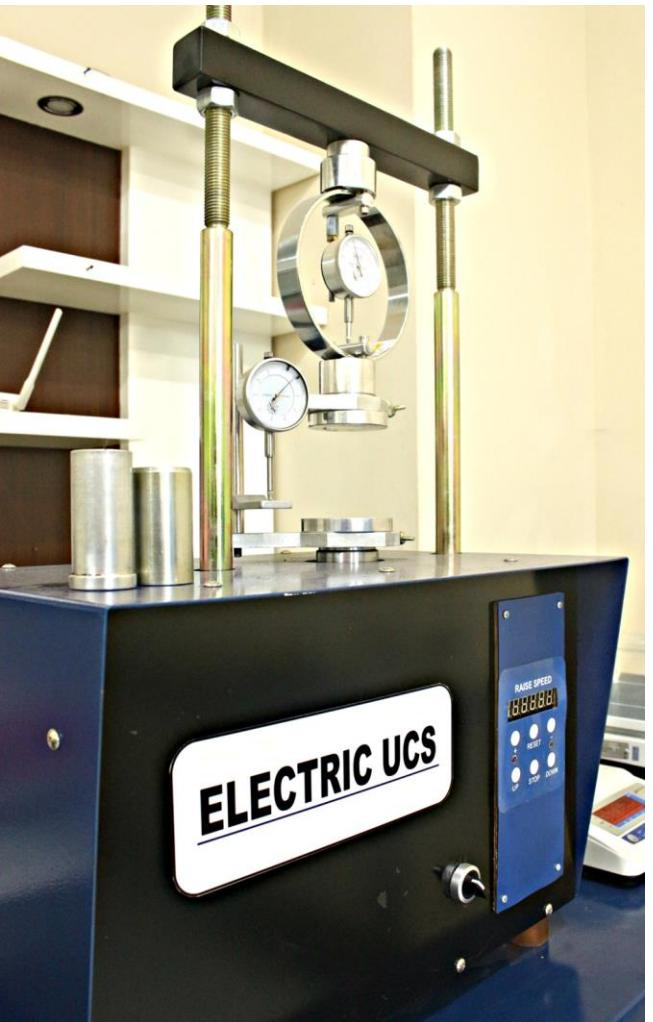
The unconfined compression test (ASTM D2166), uses a tall, cylindrical sample of cohesive soil subjected to an axial load. This load applied quickly to maintain undrained condition. The test result are often expressed in terms of the compressive strength ( $S_u$ ).
